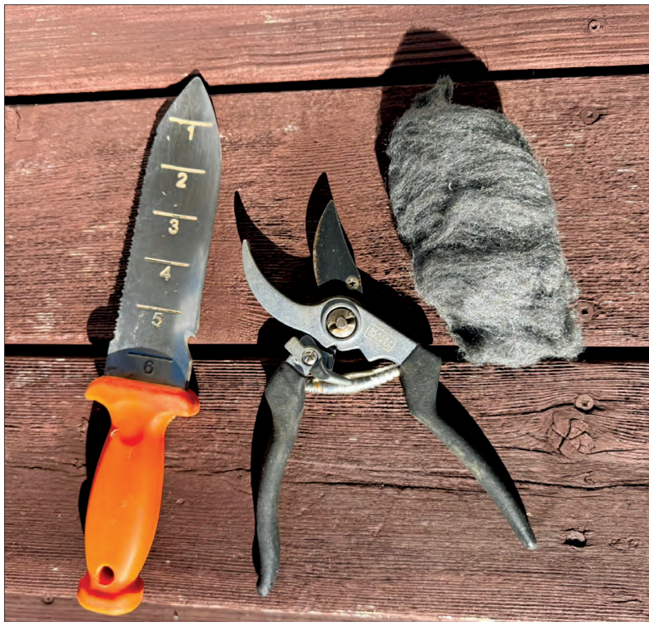
Steel wool can be used to clean debris and remove rust from your favorite garden hand tools.
