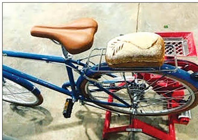
Bicycle Mill Baking uses pedal power to power their grain mill.
