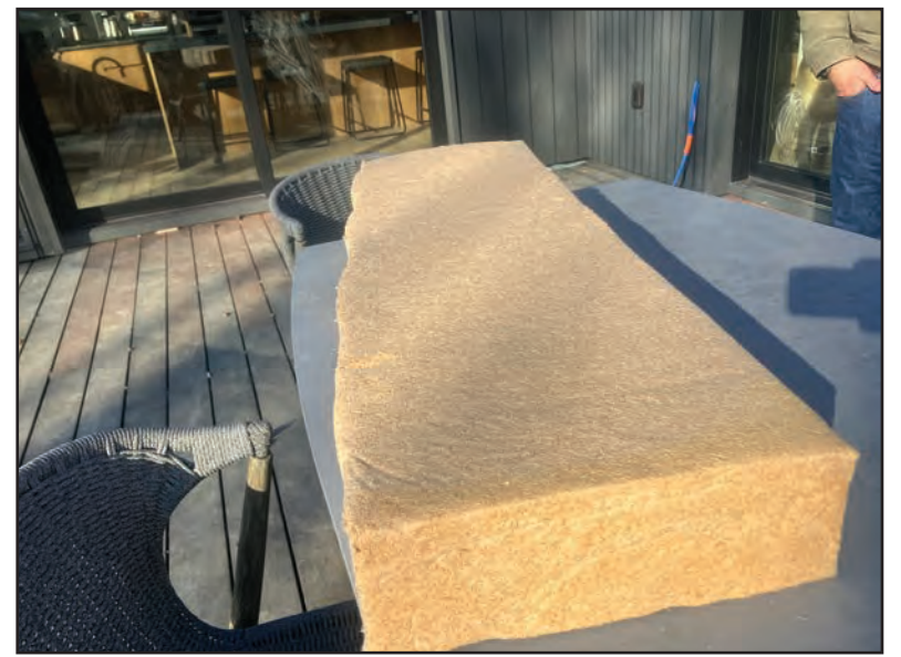
AN ADDITION ON the west side of the Weybridge house required installation of a new steel-frame staircase, above, lit by a masterfully installed “bent window” that follows the wall up above the roofline. Wood fiber insulation, shown below, along with cork insulation makes the house super energy efficient.
